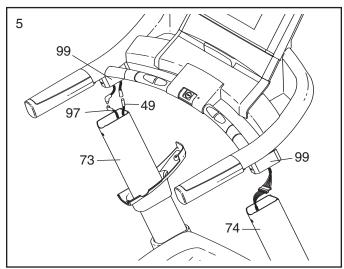
Finger tighten three Handrail Bolts (64) with three Star Washers (90) into the Right Upright (74). Next, finger tighten three Handrail Bolts with three Star Washers (not shown) into the Left Upright (73). Then, firmly tighten the six Handrail Bolts.
